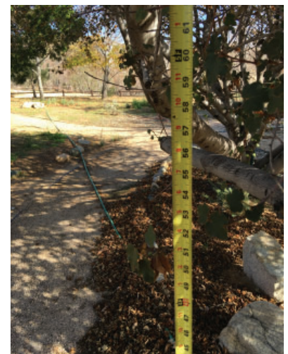
Leaf litter and garden hose on trail surface at Gilman Ranch provide trail width non-compliance; low branches from tree cause overhead obstruction
